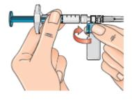
16 - Next, hold the blue vial adapter with the attached vial and remove it from the syringe by twisting it and then pulling it down, away from the syringe.
