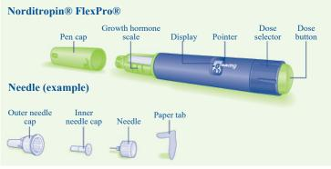
Your Norditropin® FlexPro® pen is a pre-filled growth hormone pen. Norditropin® FlexPro® contains 15 mg human growth hormone solution and delivers doses from 0.1 mg to 8.0 mg, in increments of 0.1 mg. Norditropin® FlexPro® is designed to be used with NovoFine® or NovoTwist® disposable needles up to a length of 8 mm.
